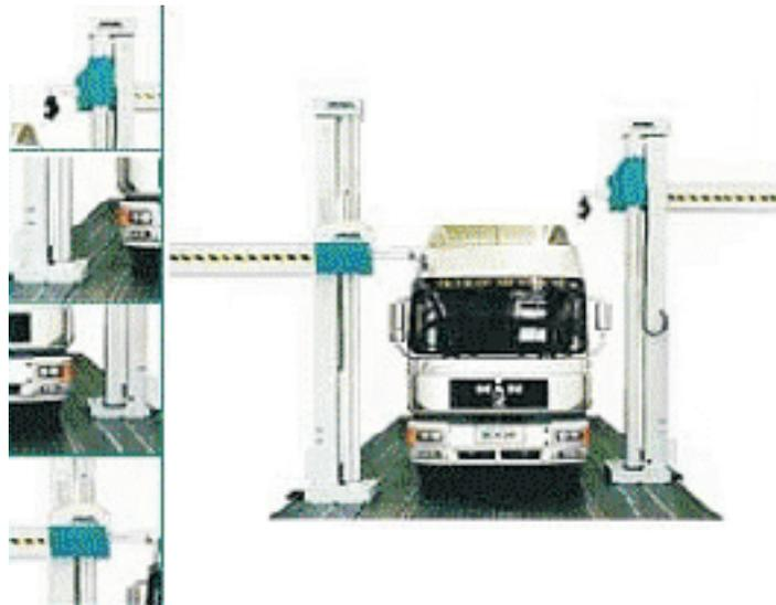
**Fig. 7.3** Horizontal CMM on inspection work
