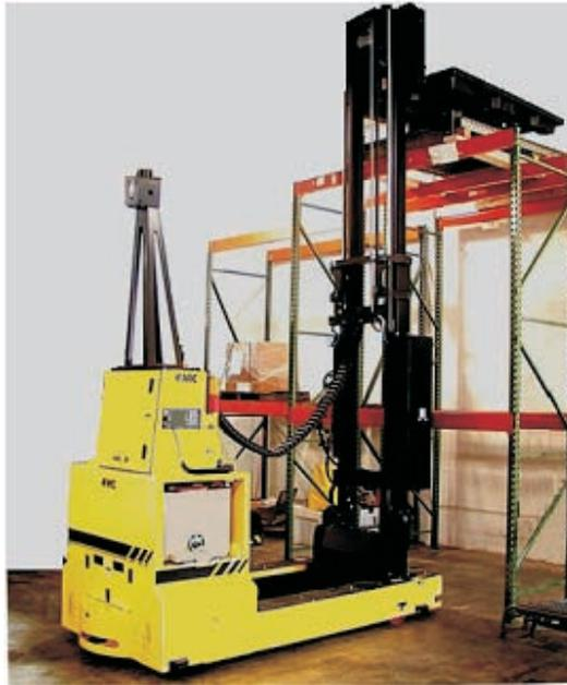
**Fig. 8.1** Reach type (automated guided vehicle)
