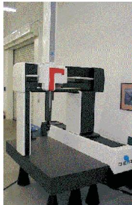
**Fig. 7.9** DCC (Direct Computer Control) CMM
